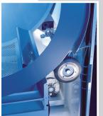
Some dryers use the same type of drive and support as 400 lb. dryers. There's no maintenanceprone gear box either. (Feature available on M96, M122, M175, M190 and M202.1
